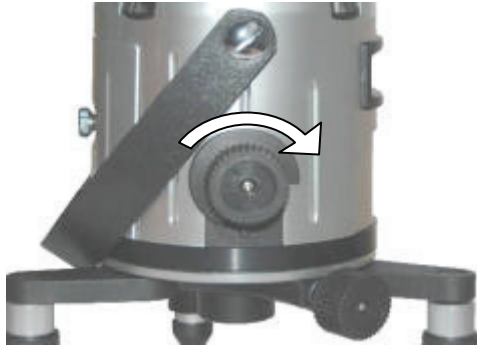
“LOCK” status, turn according to the arrow direction to unlock the unit
